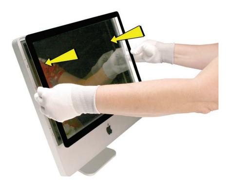
13. Clean the outside of the glass panel with a clean microfiber cleaning cloth. If necessary, spray a small amount (two pumps) of iKlear polish on the outside of the glass panel. Wipe the glass until the solution completely disappears and there is no longer any residue or haze. CAUTION: Do not use single wipe iKlear packets or other cleaning solutions to clean the glass.
